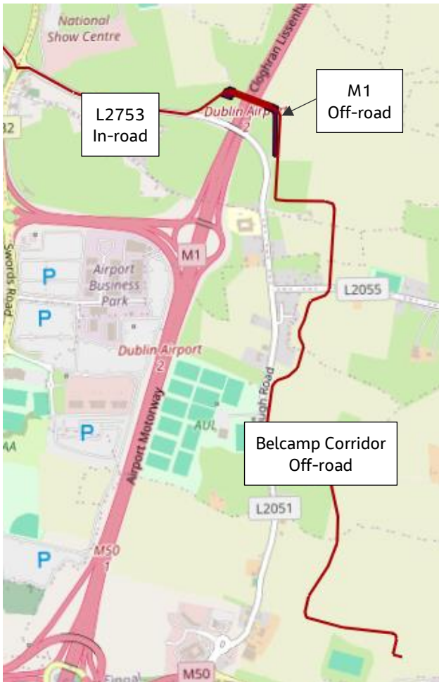
Image 4.11: Proposed Cable Route Along the L2753 Local Road, across the M1 Motorway to Belcamp Substation
